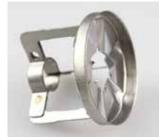
AIR NOZZLE If the air nozzle is extremely sooty, the burner has been affected by a lack of ventilation and it requires changing.
